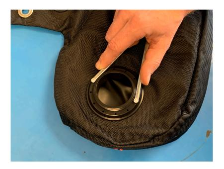
2. Replace inner bladder - unzip outer cover and remove polyurethane inner bladder. Install 420D nylon bladder and follow same procedure for reinstallation of retaining ring
